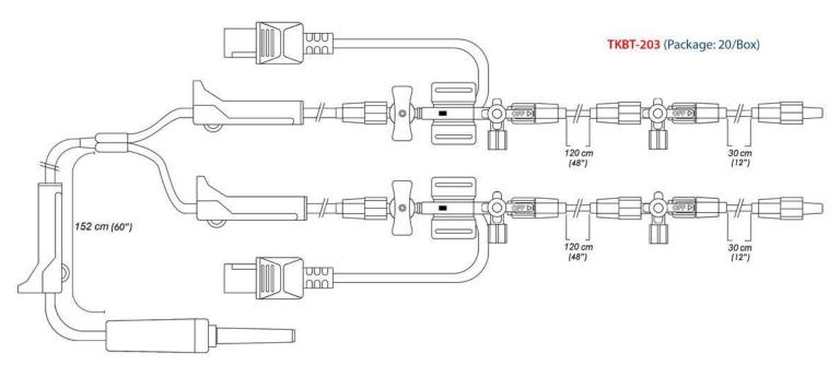
Double Channel Disposable Pressure Transducer Set, (2 pieces Disposable Pressure Transducer, 1 piece 152 cm (60") Single IV set, 2 pieces Flush Device 3 cc/h, 2 pieces 120 cm (48") Pressure Tubing with M/F Connector, 2 pieces 30 cm (12") Pressure Tubing with M/F Connector, 4 pieces 3-Way Stopcock, 4 pieces Male Non-Vented Cap).
