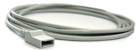
FMT IBP Cables are for connection between disposable or reusable transducers and the specified monitoring system. All cables are 3.5 m (11') in length and packaged individually. Cables are reusable, non-sterile and can be EtO gas sterilized a limited number of times. Please see FMT IBP Cables product catalogue for compatible monitors.
